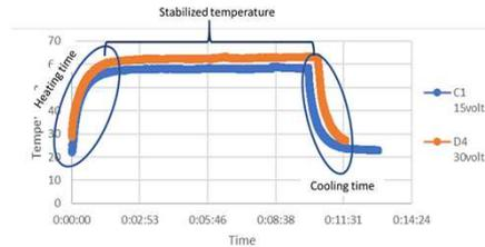
Figure 6. For all carbon formulations, when the appropriate voltage is applied, the temperature increases quite fast, stabilizes and decreases very fast when the voltage is switched off.
