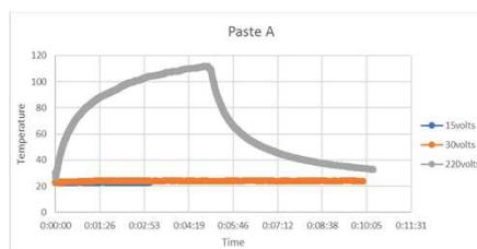
Figure 4. Paste A, due to its high resistivity value, needs high voltages to increase the temperature. An increase of 100°C is registered in 4 minutes when 220V were applied
