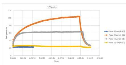
Figure 3. Chemical composition of pastes is a key parameter in the thermal behavior stabilizing the temperature values. Pastes B, C and D increase temperature applying 15volts, whereas paste A is not heated at this voltage.
