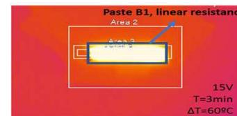
Figure 2. The thermographic analysis shows that samples are uniformly heated along the linear resistance
