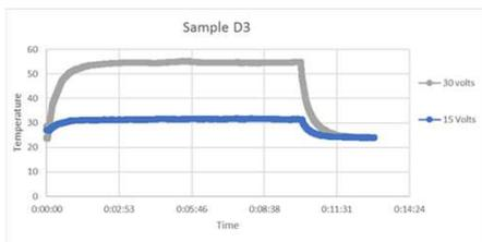
Figure 5. Temperature increases until a stabilized temperature determined by the chemical composition of the paste and the voltage applied. The figure shows the voltage influence.
